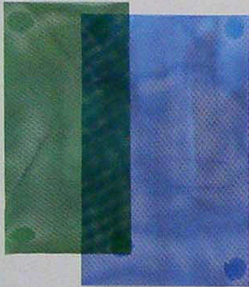
ART AREA 3.1 ADULT READING ROOM SAMPLE PAINTED 0.8 MM POLYESTER MOSQUITO NETTING FABRIC
